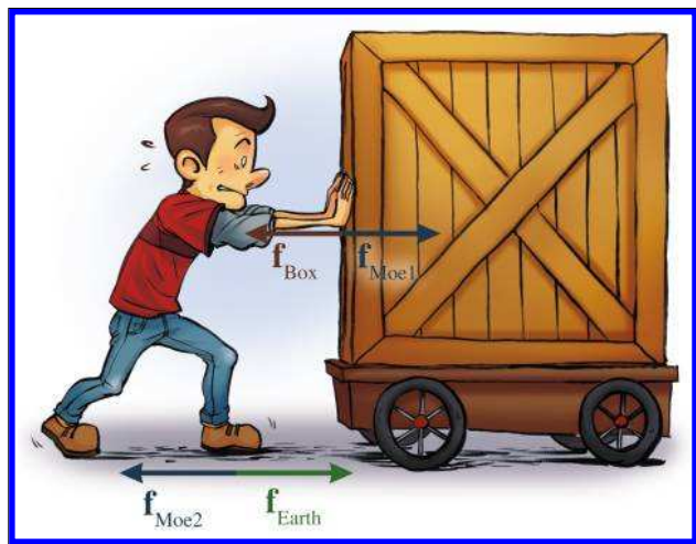
Figure 12.3 The four forces involved in Moe pushing the box
